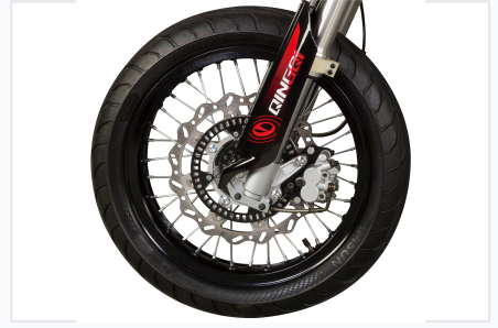
Big diameter front floating disk brake for superior stopping power.
