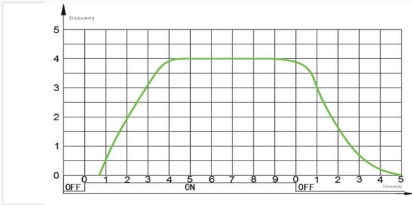
Performance graph showing the actuator stroke reaching 4mm within 4 minutes of operation.
