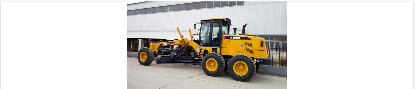
Heavy-duty 215 HP motor grader designed for road maintenance and leveling.
