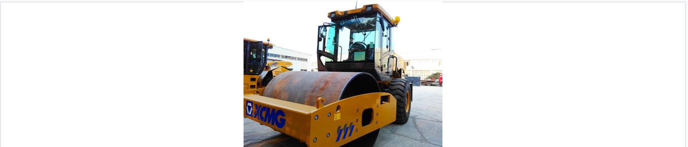
Heavy-duty single drum road roller in operation.
