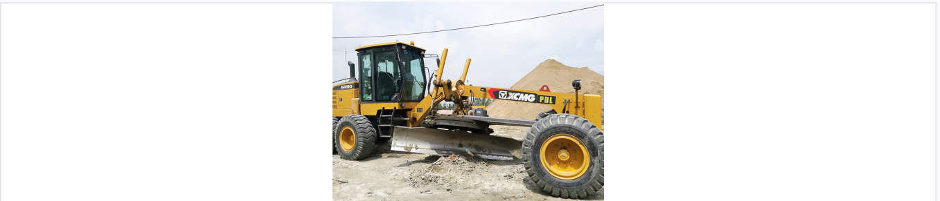
Articulated frame design for high maneuverability on construction sites.
