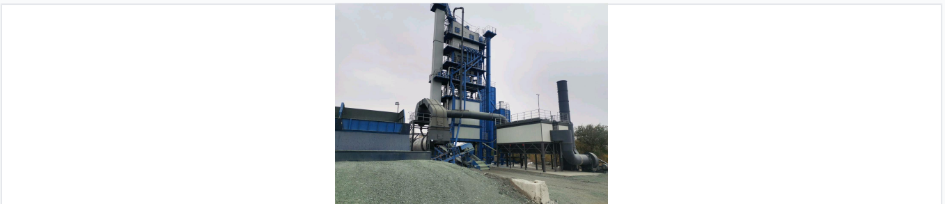
Complete overview of the QLB2000 asphalt mixing plant, showing the aggregate bins, drying drum, and mixing tower.
