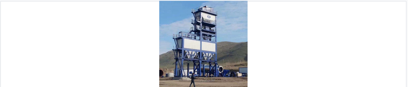
A comprehensive view of the stationary asphalt production unit including drying and mixing modules.
