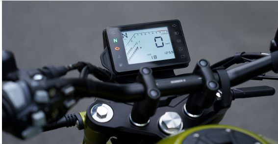
Digital instrument cluster with ABS and gear indicators.
