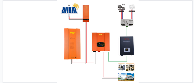
Complete system setup showing battery pack connectivity with PV panels, grid, and household appliances.
