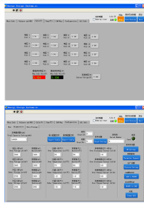
Real-time monitoring software showing individual cell voltages and system protection parameters.
